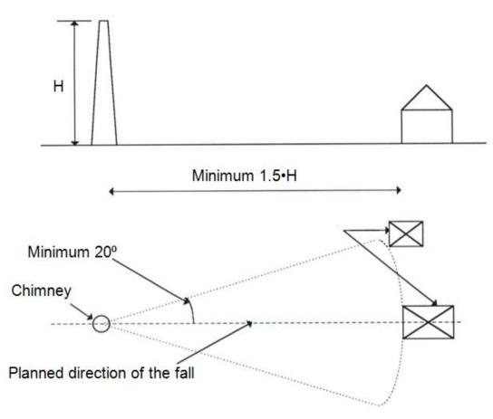
Safety distance to neighbouring buildings due to the impact of the chimney on dry ground. It should be noted that it may be necessary to protect windows and facades with wooden boards or suspended fabric covers.
