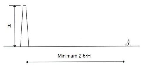
Safety distance in the direction of the fall to unprotected persons/bystanders as a result of the impact of the chimney on dry ground.
